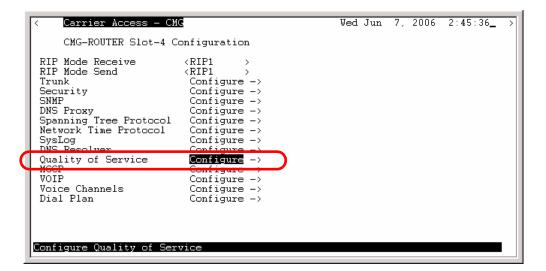
2. To enable Quality of Service, scroll < Disabled > to < Enable >, with the [SPACEBAR], select [ENTER].
